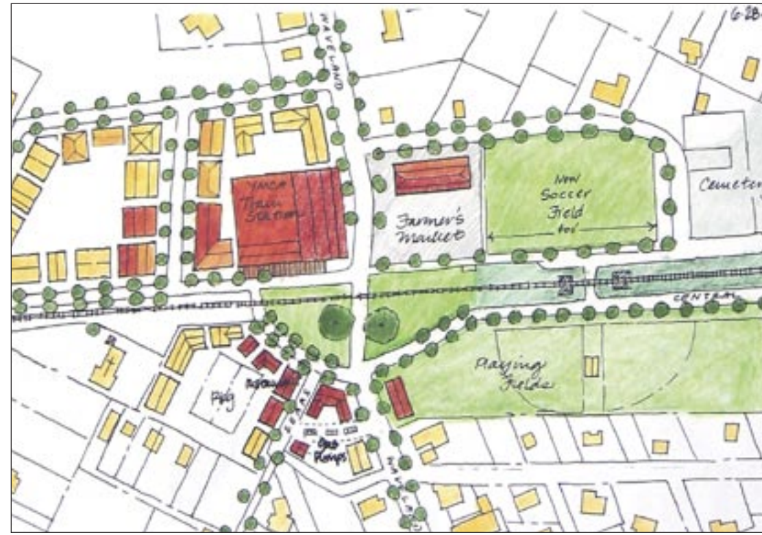
Proposed Plan: crank Central Ave slightly southward, allowing more room for Waveland Avenue to cross the railroad. Create a little green here for new buildings to face.
