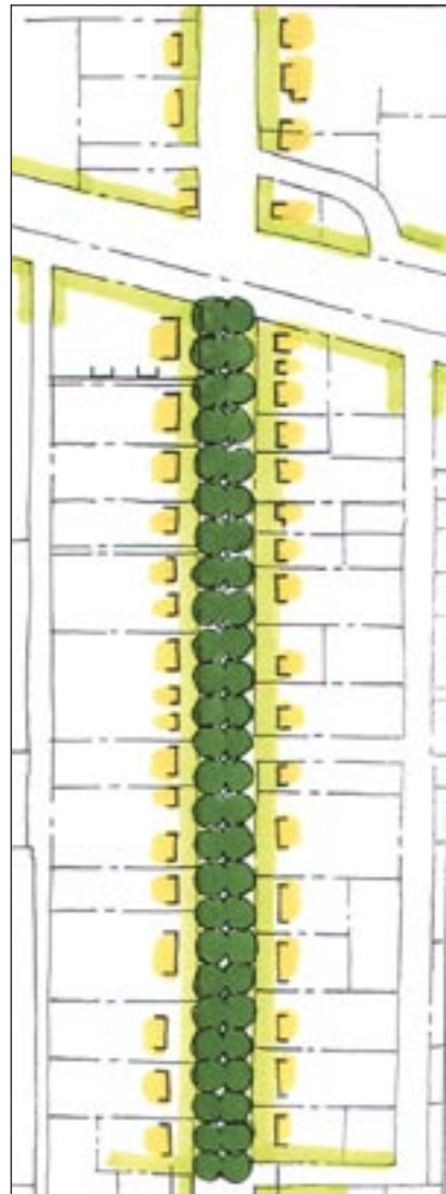
Proposed Plan of Nicholson Ave. showing a 100' right-of-way and 30' setbacks on either side.
