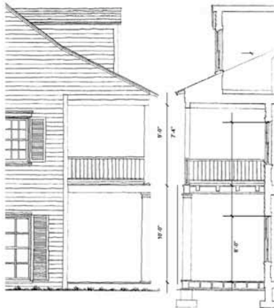
Partial elevation and wall section
